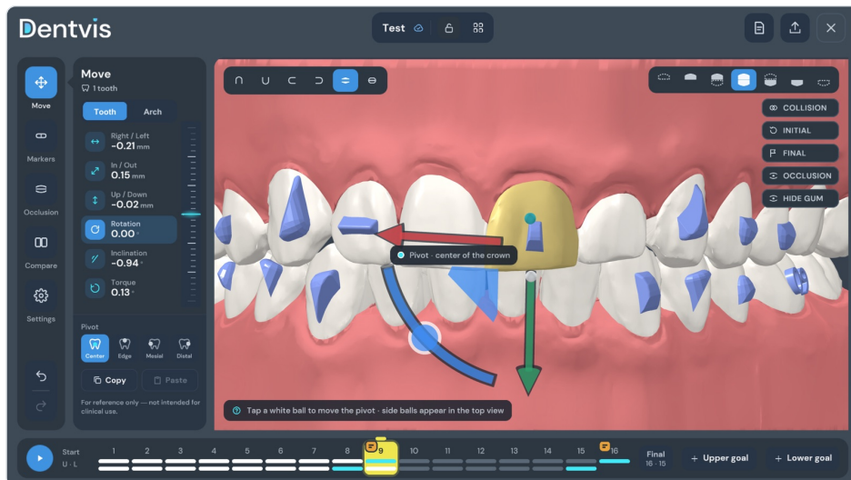
Figure 16. Move — gizmo with arrows and rings, pivot at the center of the crown, values in the panel.
