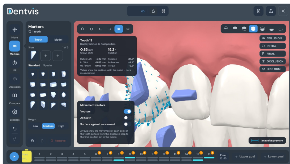
Figure 21. Markers → Tooth — the card Movement vectors : arrows on the crown of the selected tooth, the summary from the displayed step to the final position and the scale 1 mm of movement .
